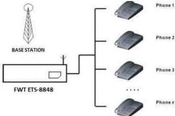
**Draw your attention:** Because there are many types of ordinary telephone and their electric parameters are different. In order to avoid mutual disturbance between telephone and terminal and affect voice quality. The distance between telephone and terminal is 1.5m at least.
